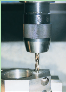
1 Drill coolant passage, leaving reaming allowance.
