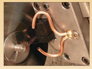
TwinPop nozzle shown installed in lathe turret.
