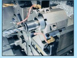
**JetTubes** shown on CNC turning center.
