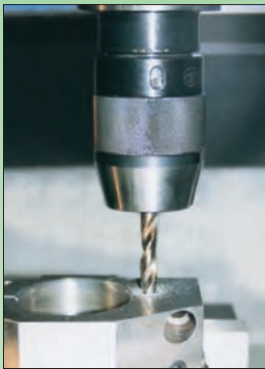
1 Drill coolant passage, leaving reaming allowance.
