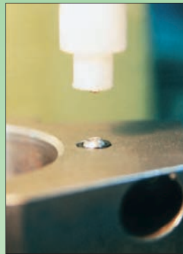
3 Press in JiffyJet until body is flush.
