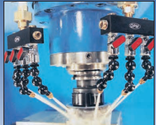
QPM Manifolds enable 6 SwivelMax nozzles (see page 20) to be used in this face milling operation.
