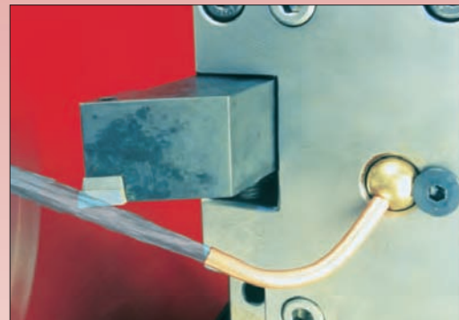
LolliPop nozzle shown installed in lathe turret.
